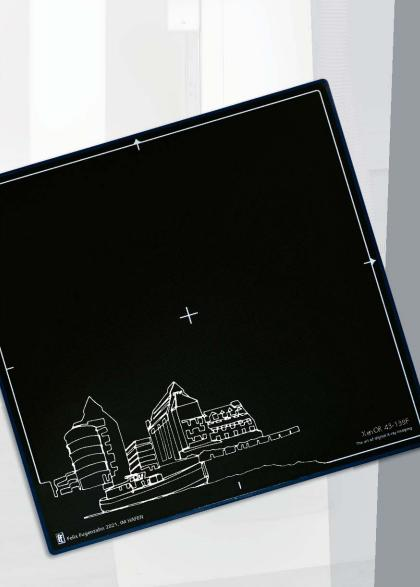
With Auto Exposure Detection (AED) detection and a low weight, the cable-connected CsI X-ray detector XenOR 43-139F in cassette format is ready for a wide range of applications in digital radiography. The detector can be used, for example, for retrofitting existing X-ray systems. It has 139  $\mu$ m resolution and 16-bit ADC for more image detail. It is the optimal choice for a high-endend DR system.
